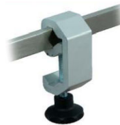
USU-02 Vice-type holder 96 × 40 mm · rail 25–40 mm, pipe Ø 20–40 mm
